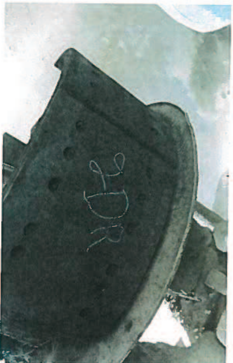
Sabot freins 2ieme ess.dr. (13mm)
