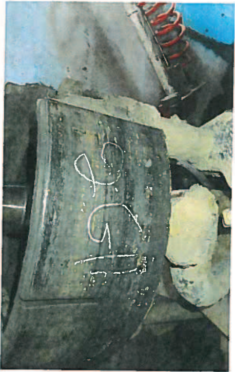
Sabot freins 2ieme ess.g. (12mm)
