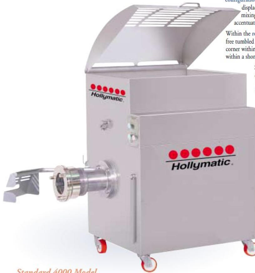
Standard 4000 Model 20hp - 2 Speed Grind Motor - 56 Cutting Head with Stainless Steel barrel, Feedscrew and Aluminum Bronze Lock Ring
